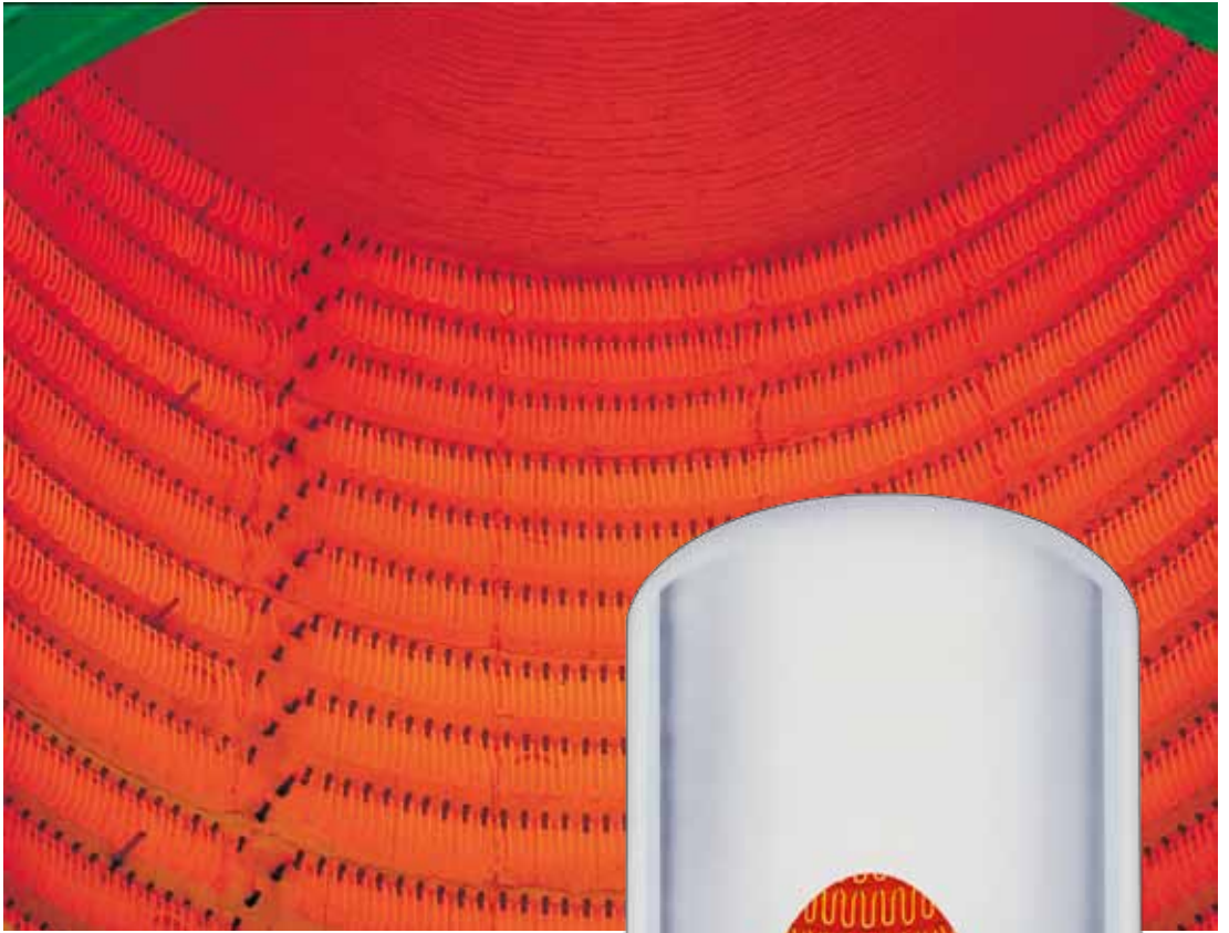
Fig. 22 ROB-modules in a bell furnace.
