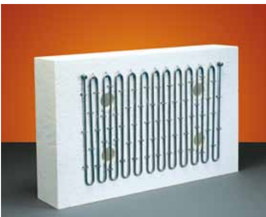
Fig. 3 Fibrothal meander II module with free-radiating heating elements for a maximum element temperature of 1300°C (2370°F), mainly for roof heating and tilting furnaces.
